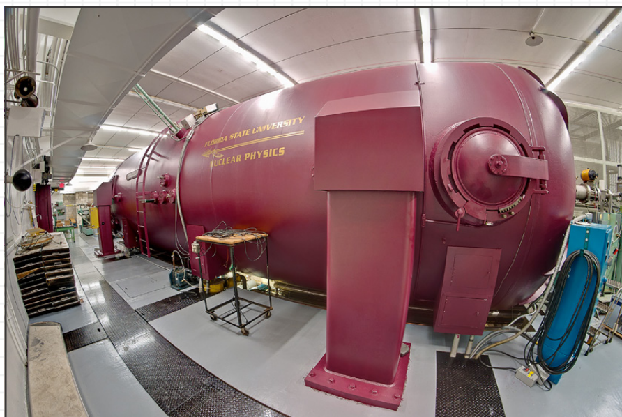
The 9-MV Super-FN Tandem van-de-Graaff accelerator in FSU's John Fox Laboratory.
